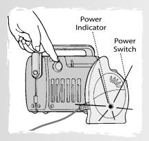
Place transmitter in room in which you intend to use it. Rotate transmitter power switch to turn power on. Power indicator lights. Turn on a radio.
